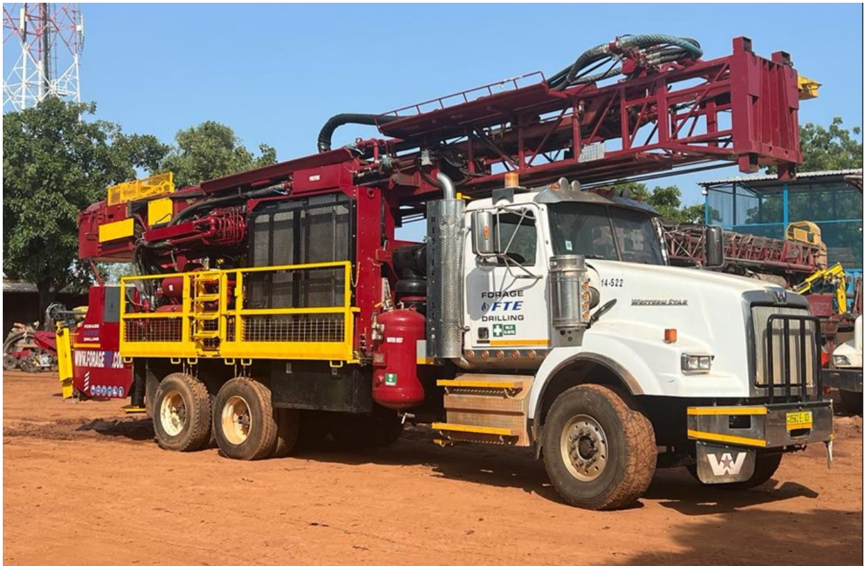
Picture 1. Forage FTE Drilling's RC Drilling Rig
